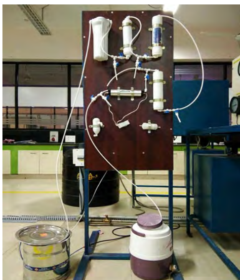
Fig. 1 Experimental setup of coconut water collection unit
