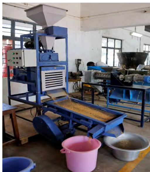
Fig. 2. Performance evaluation of the developed decorticator for foxtail millet
