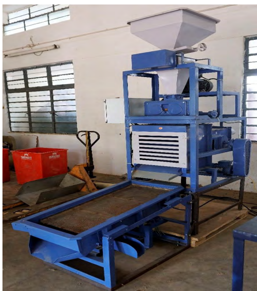
Fig. 1. Decorticator for foxtail millet
