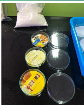
9 cm disc of packaging material inserted into petri dish
