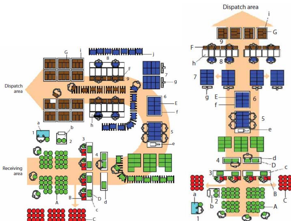
Fig. 1.11: U type configuration and Straight line configuration of mango packing house (FAO, 2012) (1) Maturity test, (2) weighing, (3) sorting and trimming, (4) delatexing, (5) hot water treatment, (6) cooling, (7) air-drying, (8) sizing, (9) packing. Equipment: (a) flotation tank, (b) weighing scale, (c) sorting table, (d) delatexing tank, (e) hot water tank, (f) cooling tank, (g) fans, (h) sizing table, (i) pallets. Materials: (A) full baskets, (B) reject fruit, (C) empty baskets, (D) full crates, (E) treated fruit in crates, (F) empty cartons, (G) full cartons
