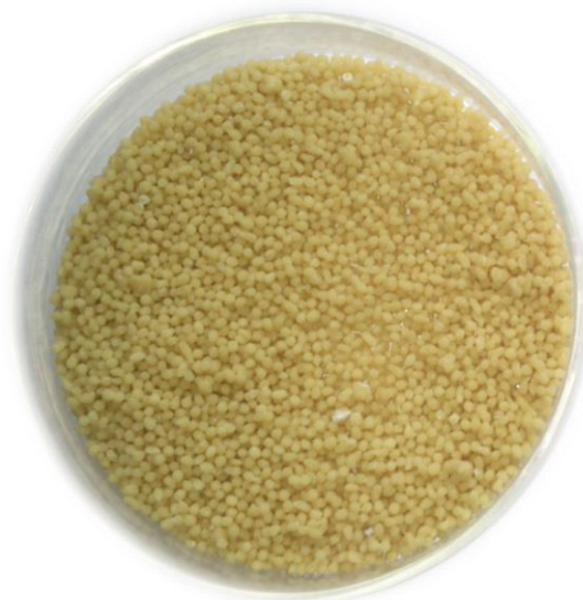
Fig: Beads of alginate, whey protein and fish oil coated with high melting fat
