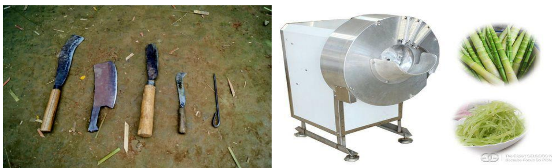
Fig. 5.6: Bamboo shoot Cutter (Manual and mechanical equipment)
