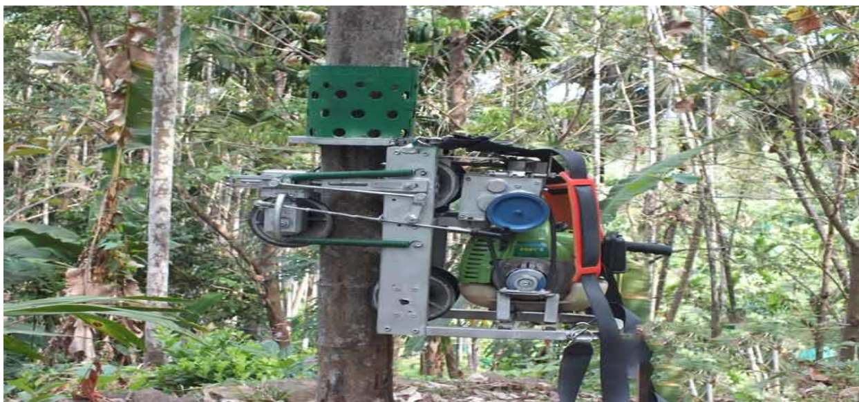
Fig. 5.2: Automated Arecanut Climbing and Harvesting Machine
