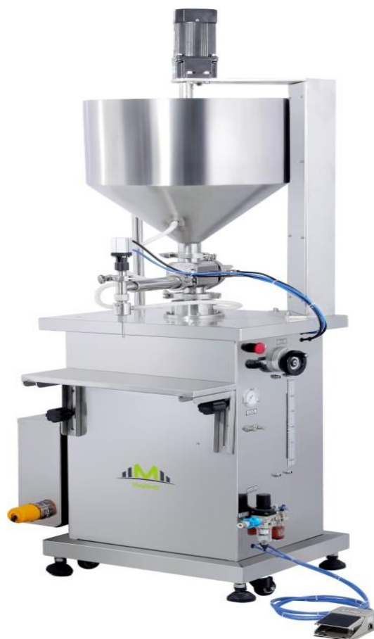
Fig. 5.12: Semi automated bottle filling machine
