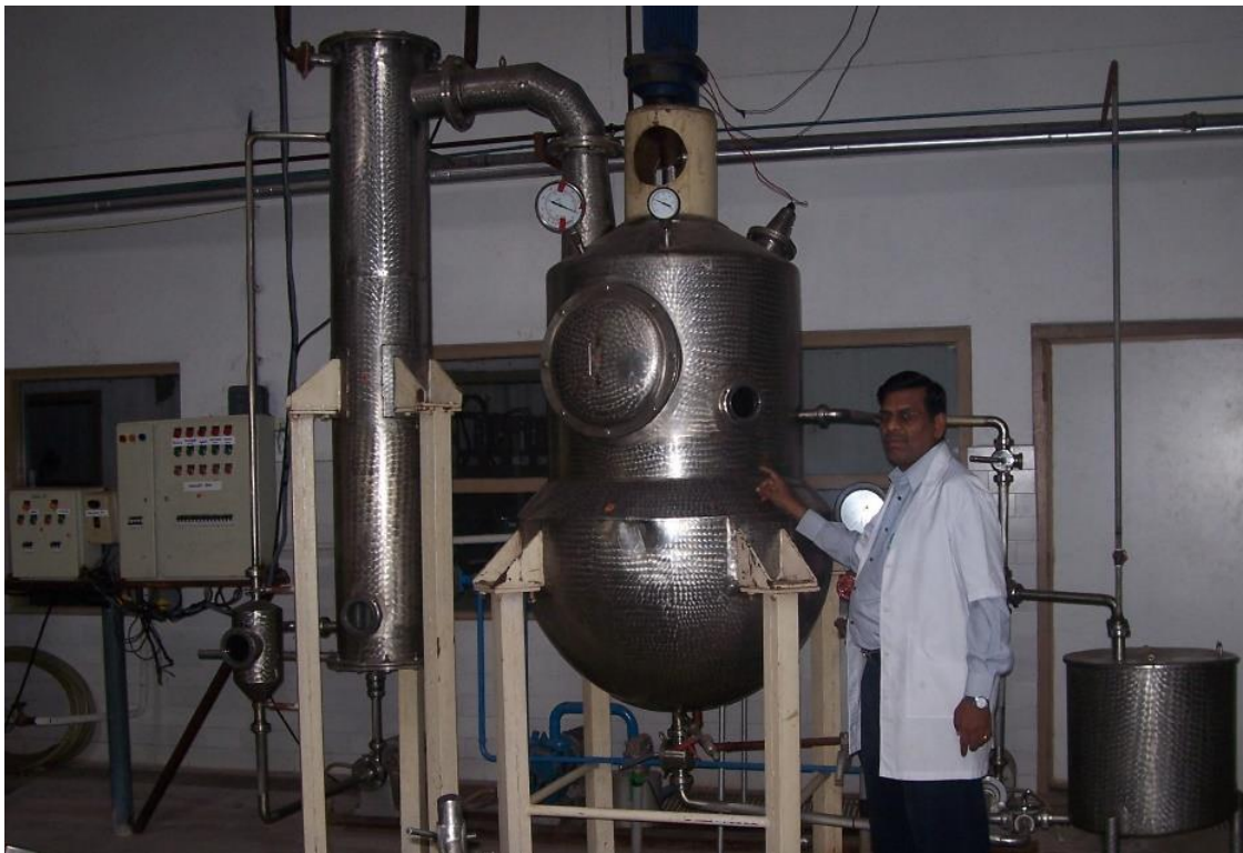
Fig. 9. Vacuum Pan (Batch Evaporator) with Condenser and controls (Courtesy: SVVU, Tirupati)
