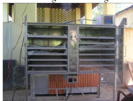
Fig.2.78: Fire wood operated drier for mace or nutmeg drying
