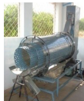
Fig.2.56: Grader for raw cashewnut
