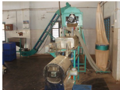
Fig. 2.65: Impact and shear type peeler
