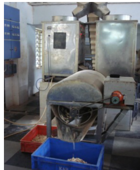
Fig.2.64: Abrasive type peeler
