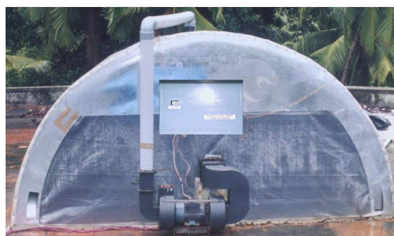
Fig. 2.3: Solar tunnel dryer with electricity as an alternate source of energy
