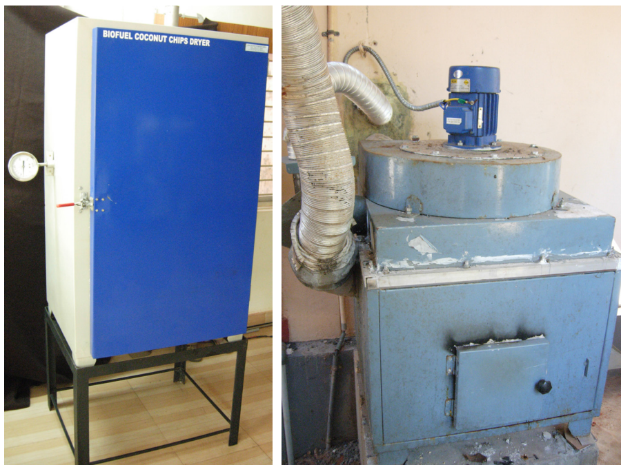
Fig.2.11: Electrical and Agricultural waste fired coconut chips dryer
