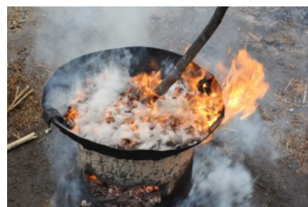
Fig.2.53: Open pan roasting of cashewnut
