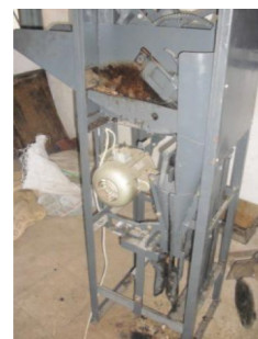
Fig.2.61: Vertical type reciprocating mechanized sheller
