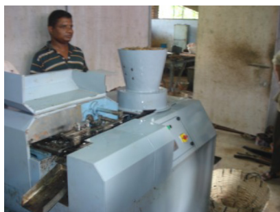
Fig.2.60: Automatic cashewnut de-sheller
