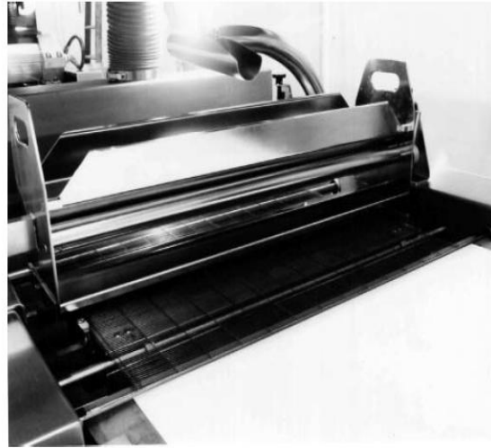
Fig. 17.2 Gravity flow pan for top coating.
