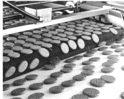
Fig. 17.9 Turn-over of half-coated (bottomed) biscuits.
